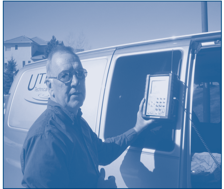
Dave Anderson of Utility Technical Services analyzes water leak results using a Leak Noise Correlator.
